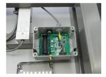
Insert the battery in the battery holder. The LED turns green for 1 second.
